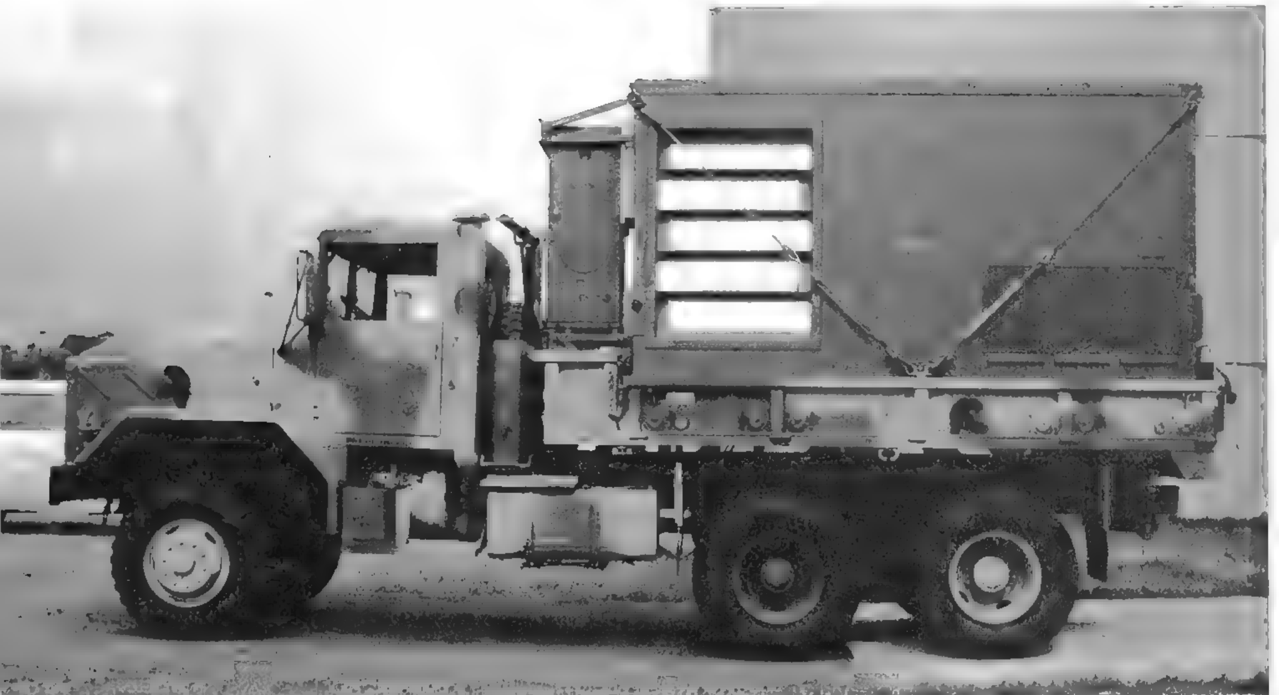
This particular M923 has an F36T4-2S shelter in its bed. Visible behind the cab, which has been fitted with the optional hard top, is the spare tire and its handling davit. (Photo courtesy of Keco Industries)
